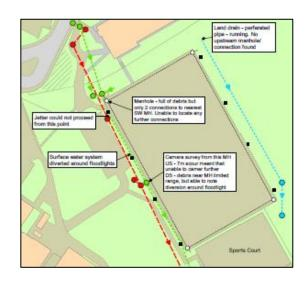
The second was traced back to a previous misconnection of foul waste from a neighbouring commercial premises to the storm water system that runs through the Sue Noake site alongside the ATP (see red dots in Diagram ---).
