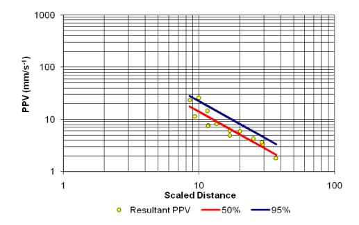
Figure 14.1 Vibration scaled distance regression model for test blast 1 and 2
