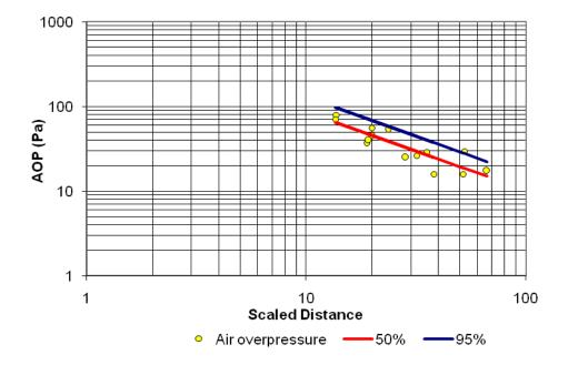
Figure 14.2 Air overpressure scaled distance regression model for test blast 1 and 2
