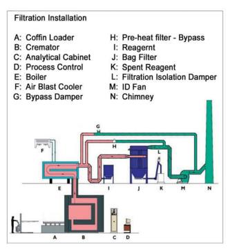
Hot gases leaving the cremator are cooled to around 120°C by passing through a Flue Gas Cooler (E) filled with a glycol/water mixture which is continuously circulated through an Air Blast Cooler (F) to dissipate excess heat to atmosphere.
