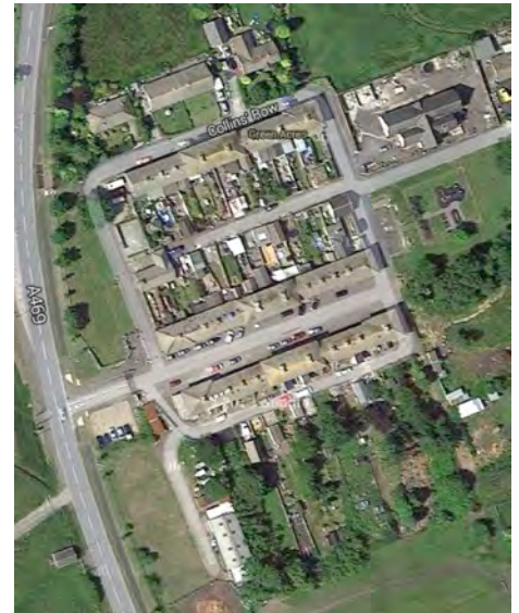
Aerial view of Bute Town showing the orthogonal grid iron plan. ©2014 Google, Bluesky
