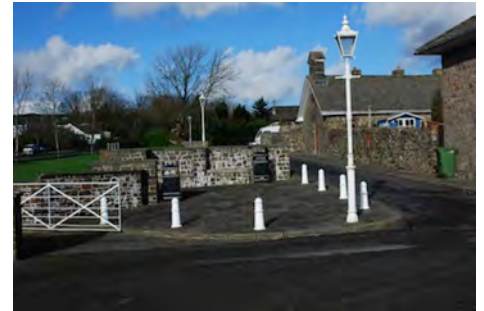
Entrance area arrangement with stark white street furniture. Note also the character of the stonework to the entrance walling is at odds with the stonework of the rows.
