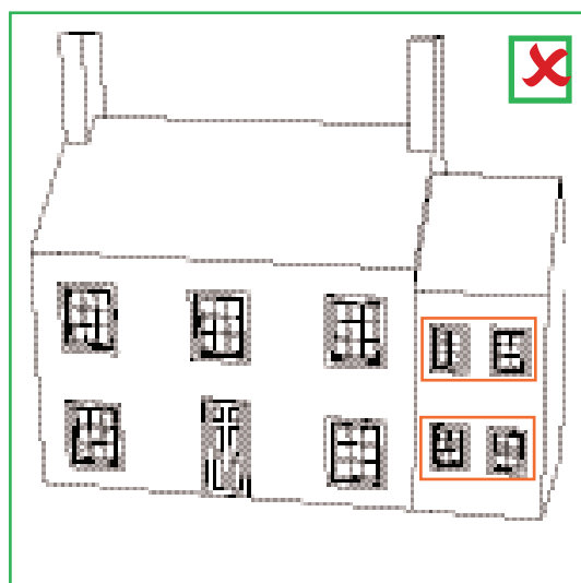
side extension: windows of wrong proportion
